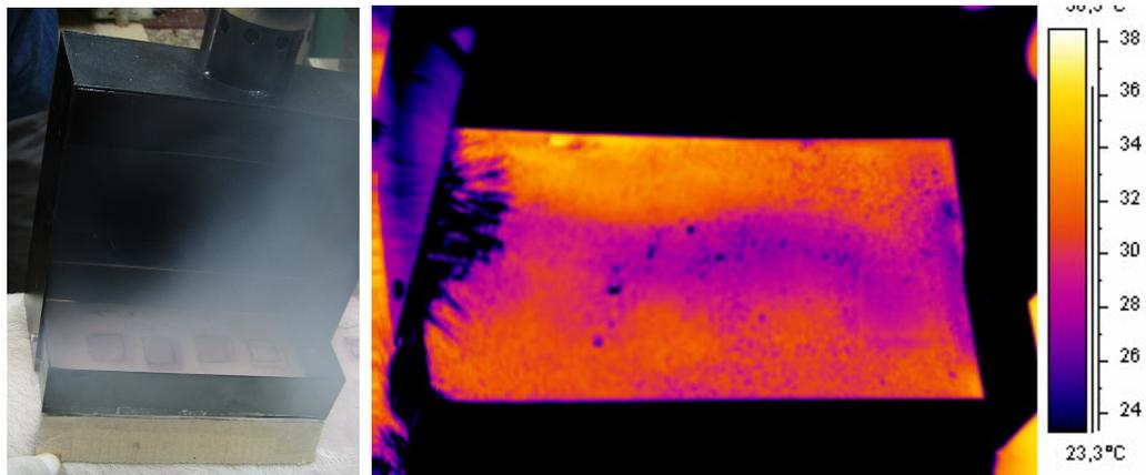
**Fig. 1.** a) Applicator used for CO<sub>2</sub> cooling procedure, b) thermal image taken at the end of the cooling phase
